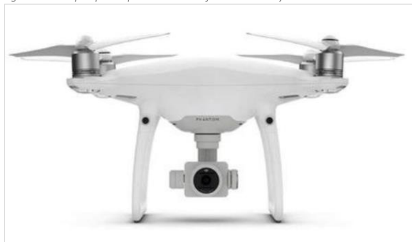
Figure 18: Sample quadcopter drone used for aerial surveys
